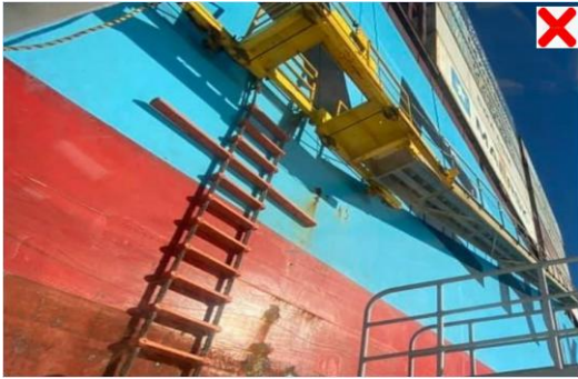
Figure 1 - Non-Compliant Trap Door Arrangement
